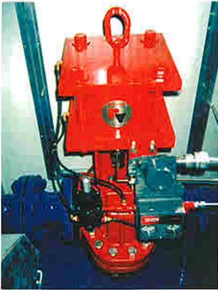
The Series 9000 High Pressure Pinch Valve features a "smart" sleeve and a "smart" positioner. As the primary gas control valve, the Series 9000 is reliable against sand abrasion.
